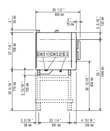
CWI1 = Cold Water inlet 1 (cleaning) CWI2 = Cold Water Inlet 2 (steam EI = Electrical inlet (power)
